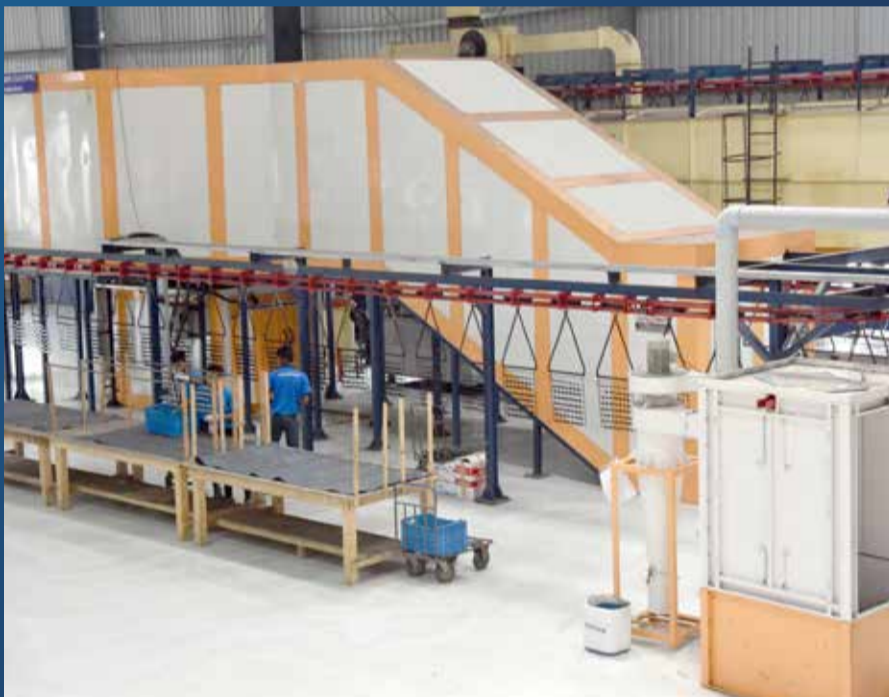
The new powder coating machine produces up to approx. 20,000 parts per shift (8 hours) at full capacity
