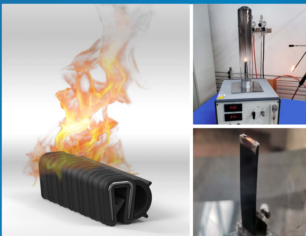
In order to meet the high requirements for gaskets in rail vehicles, EMKA uses special flame-retardant material and thus achieves the highest fire protection classes. Fire behaviour, smoke gas development and toxicity are tested in the company's own laboratory.
